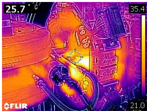
Figure 2: Temperature rise due to reduced cooling flow.
