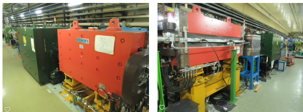
Figure 7: The beam dumps of the SuperKEKB LER and HER.
