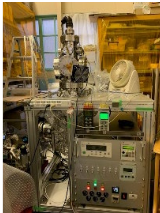
Figure 2: The evaporation equipment for oxygen-free Pd/Ti deposition.
