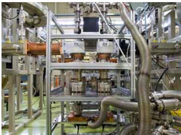
Figure 5: Photo of two couplers installed for high power test.
