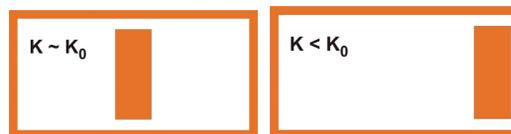
Fig. 1: Moving fin inside the waveguide we can change value of longitudinal wave vector and thus we can change the phase of wave coming through the waveguide.
