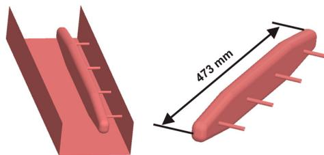
Fig. 2: Geometries of phase shifter based on WR650 waveguide and fin. Special geometry of fin provides low reflection ( $\sim -30$ dB) in all range of position.
