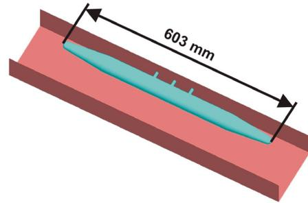
Fig. 5: Phase shifter with cylindrical shape of fin. Phase shift is  $120^\circ$ , expected breakdown power limit is 12MW.
