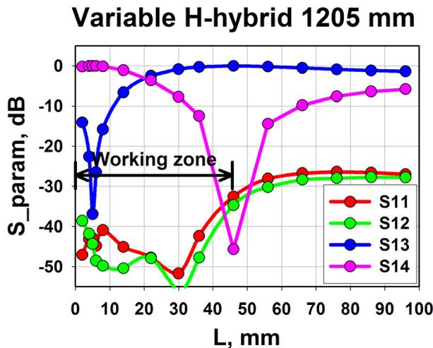
Fig. 8: S-parameters of variable hybrid with full range of coupling variation vs. fins displacement.
