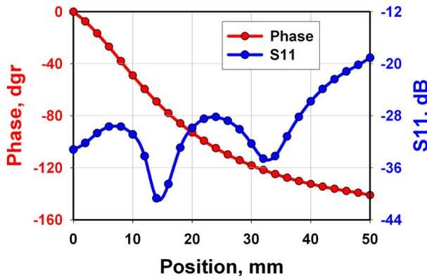
Fig. 4: Results of low power measurements of phase shifter presented at Fig.3.
