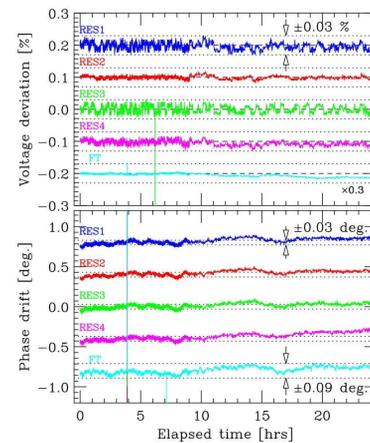
Figure 1: Amplitude and phase measured for 24 hrs.
