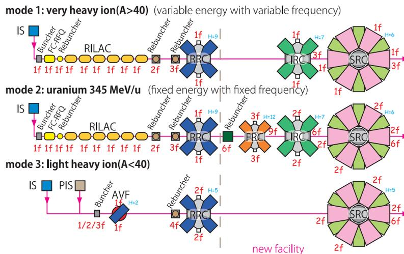
Fig.1 Acceleration modes of the accelerator complex of RIBF
