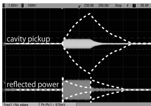
Figure 3: Profiles of the pickup signal from a cavity and the reflected power by a directional coupler on the feeder line. A full reflection occurs while the cavity voltage stopped at a certain level with a pulsed power. If we put a pulse with much more amplitude, then the cavity voltage grow up following dashed lines and reflected power is going to be zero.
