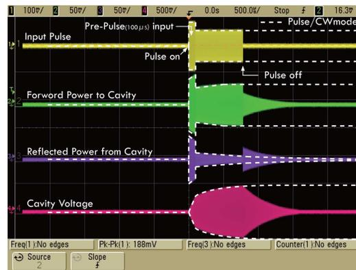
Figure 2: Pre-pulse is introduced to pulse-mode to overcome multipactor of the cavity. a) envelope of input signal to amplifier. b),c) forward and reflected power at coaxial feeder line, respectively. d) pickup signal of cavity.
