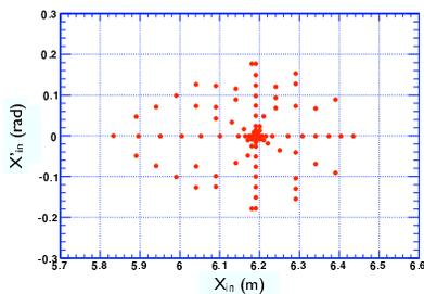
Figure 4: 97 injection points, which are used to calculate higher ordered transfer map.
