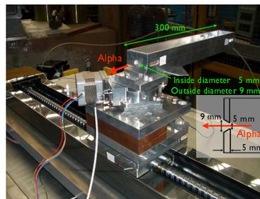
Figure 3: The alpha particle collimators on the moving stage
