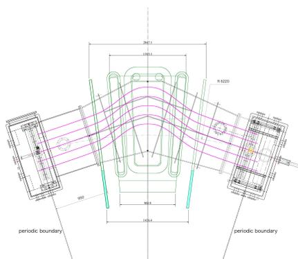
Figure 1: Experimental Setup. The alpha particle injector is on the left-hand side and the alpha particle detector is on the right-hand side. Example particle trajectories are shown in pink lines, and the PRISM-FFAG magnet is shown in green. Two holes located between the magnet and the injection chamber, and also between that and the detection chamber, are those for connecting vacuum pumps.
